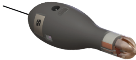
The sPAT measures 124 x 38mm (LxØ) and 60g (in air)
